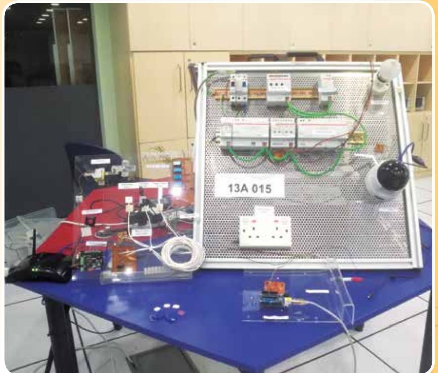
Integration of Energy Management, Fire Protection and Security features using KNX interfacing with Arduino system.
