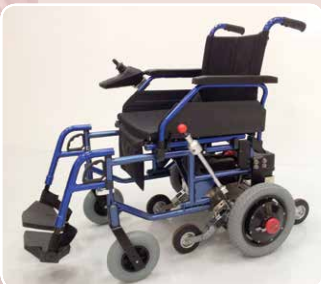
Wheelchair with gap-clearing mechanism.
