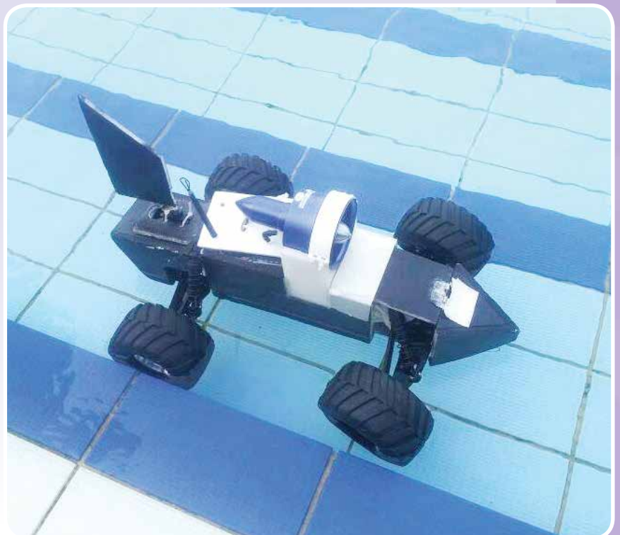
The vehicle is the first of its kind, developed on the idea of thrust propulsion.
