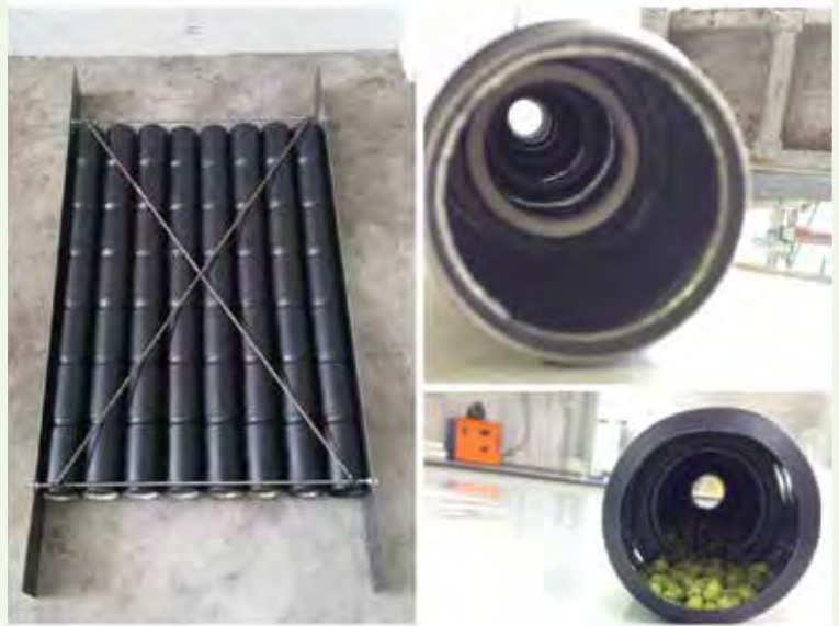
Simple and low-cost dryer to remove moisture from sorghum seeds for the community in Poncosari village.
