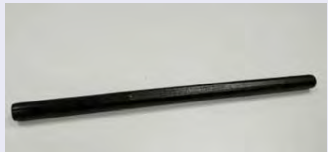
Hybrid (Braid/chopped fibre) Composite Structure with Custom Profile.
