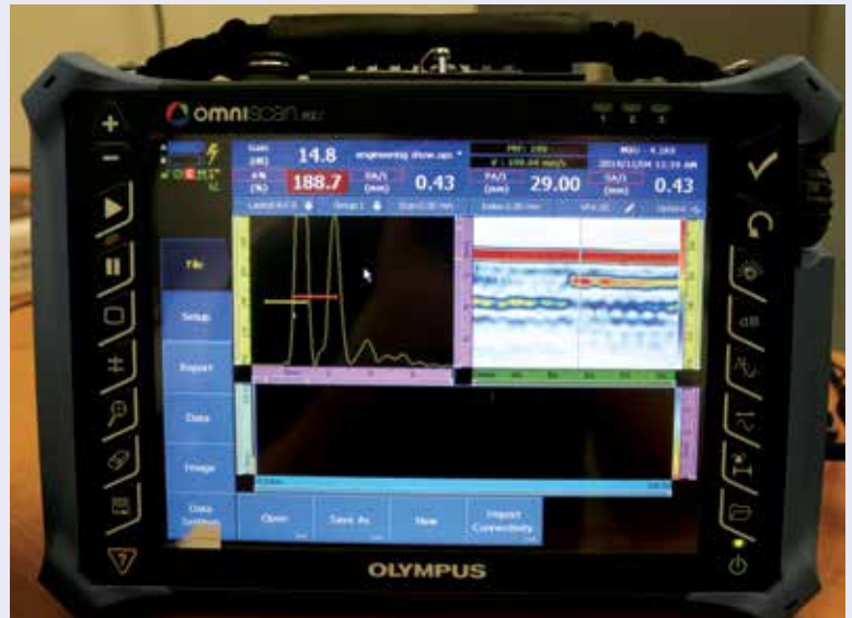
Defect in a composite panel located using phased array ultrasound inspection equipment.
