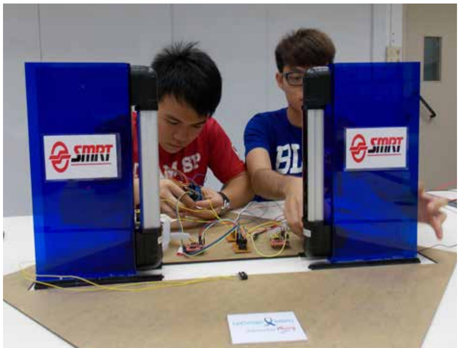
Reducing MRT door reopening, by having individually controlled doors with voice reminder to stay clear.
