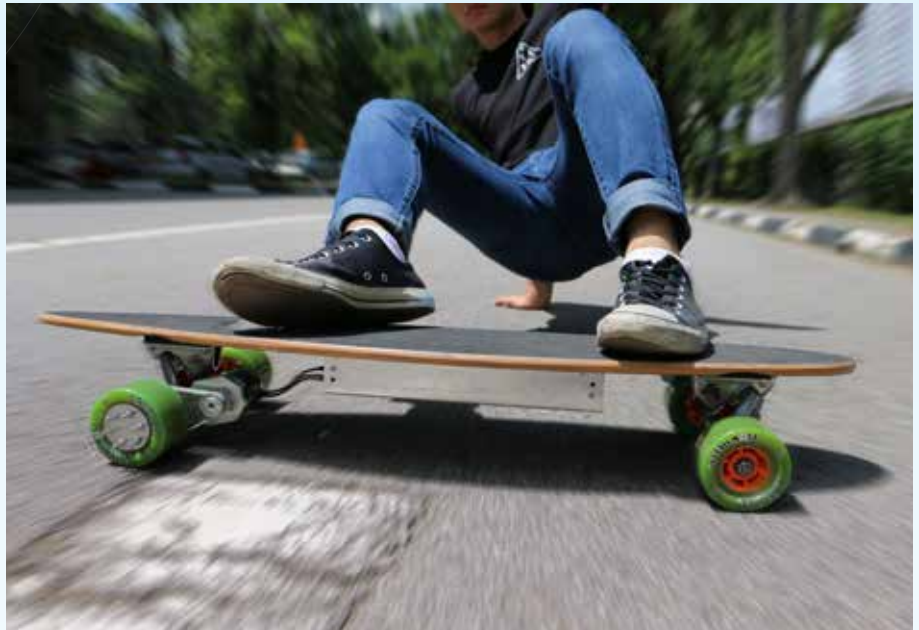
The Bazedboard in action! Electrically powered with high trucks and wheels for better control and comfort.
