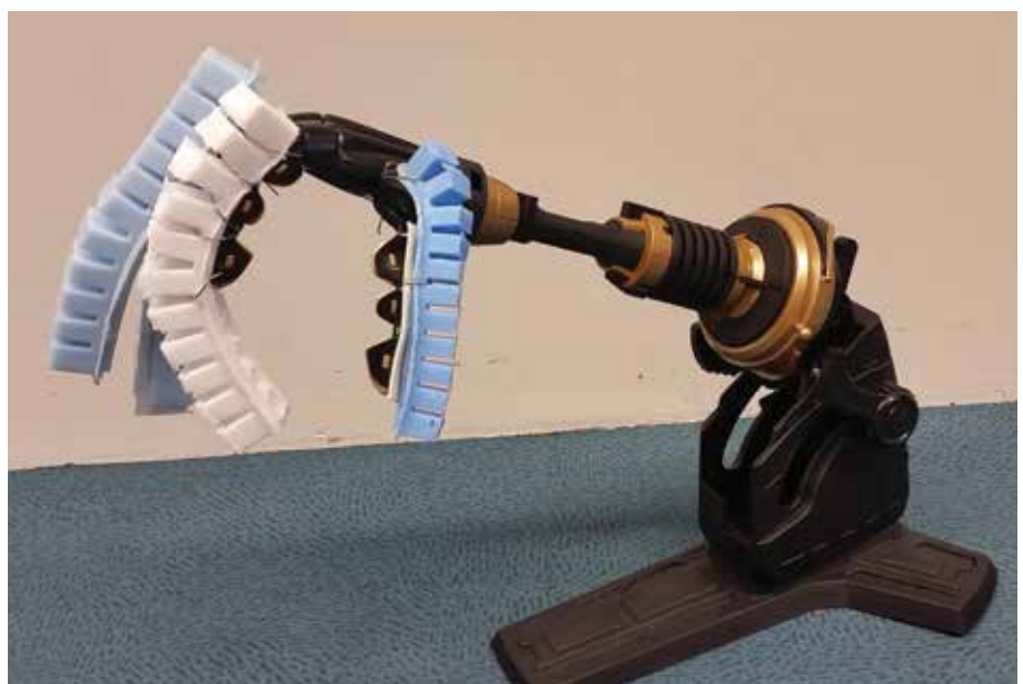
Prosthetic hand made of silicone fingers demonstrating the use of soft robotics in Assistive Technology.
