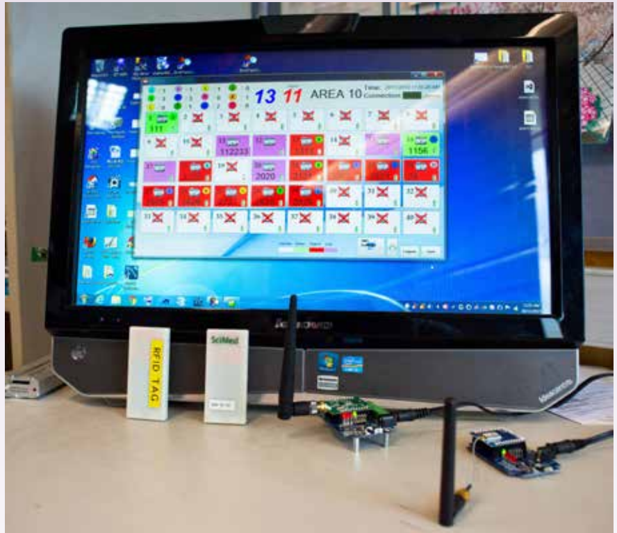
WIP Tracking System with Active RFID equipment.
