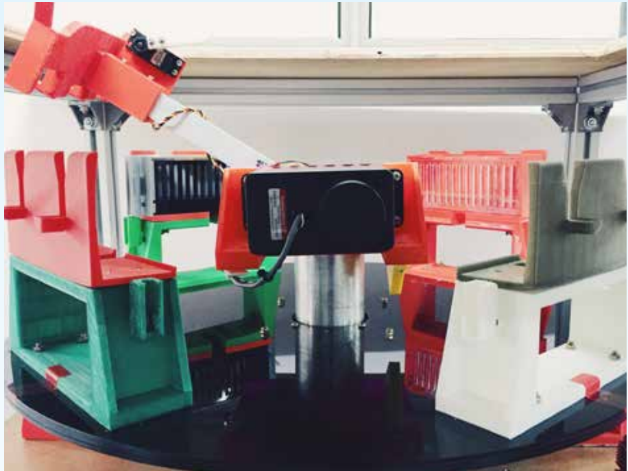
Ground battery swapping station with four battery holders and the rocker arm on the rotatable carousel.
