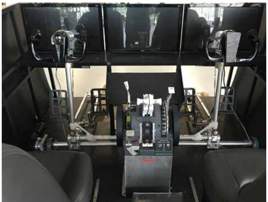
Boeing 737 Interchangeable Flight Simulator System with Flight Control Upgrades and realistic Glass Cockpit Systems.
