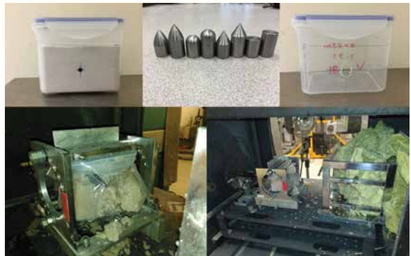
A suite of impact tests conducted with the smooth bore gas gun to determine the ballistic performance of sand.
