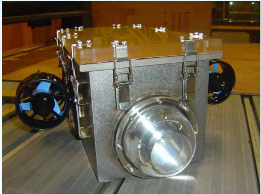
The basic compartment to house the thrusters and the controls.
