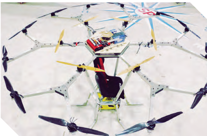
DATUM runs on a Hybrid Engine Fuel Management System with a flight time of up to 30 mins.
