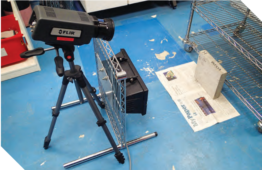
IRT setup for detection of structure defect.
