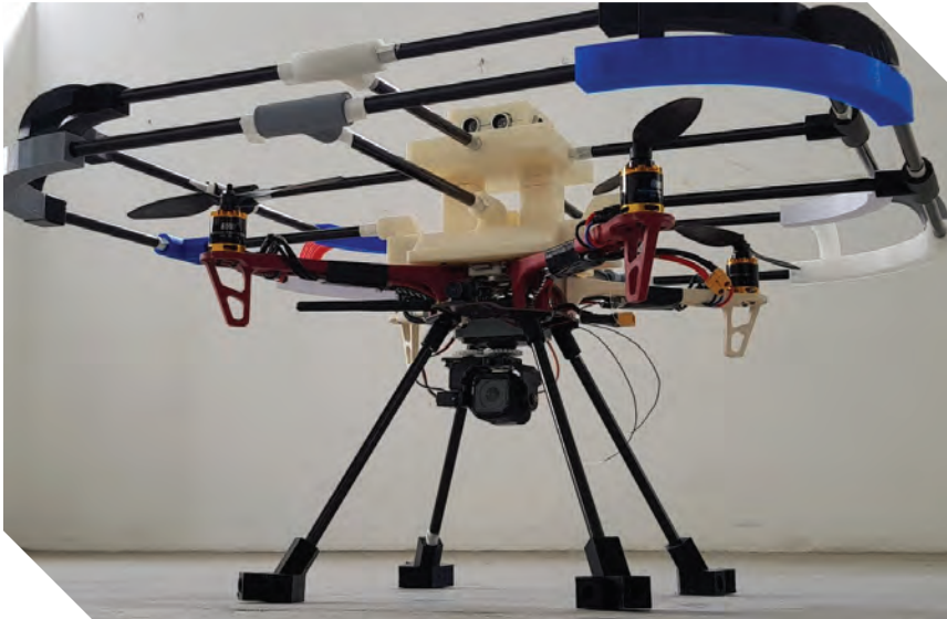
The Damage Detection Drone (D3).
