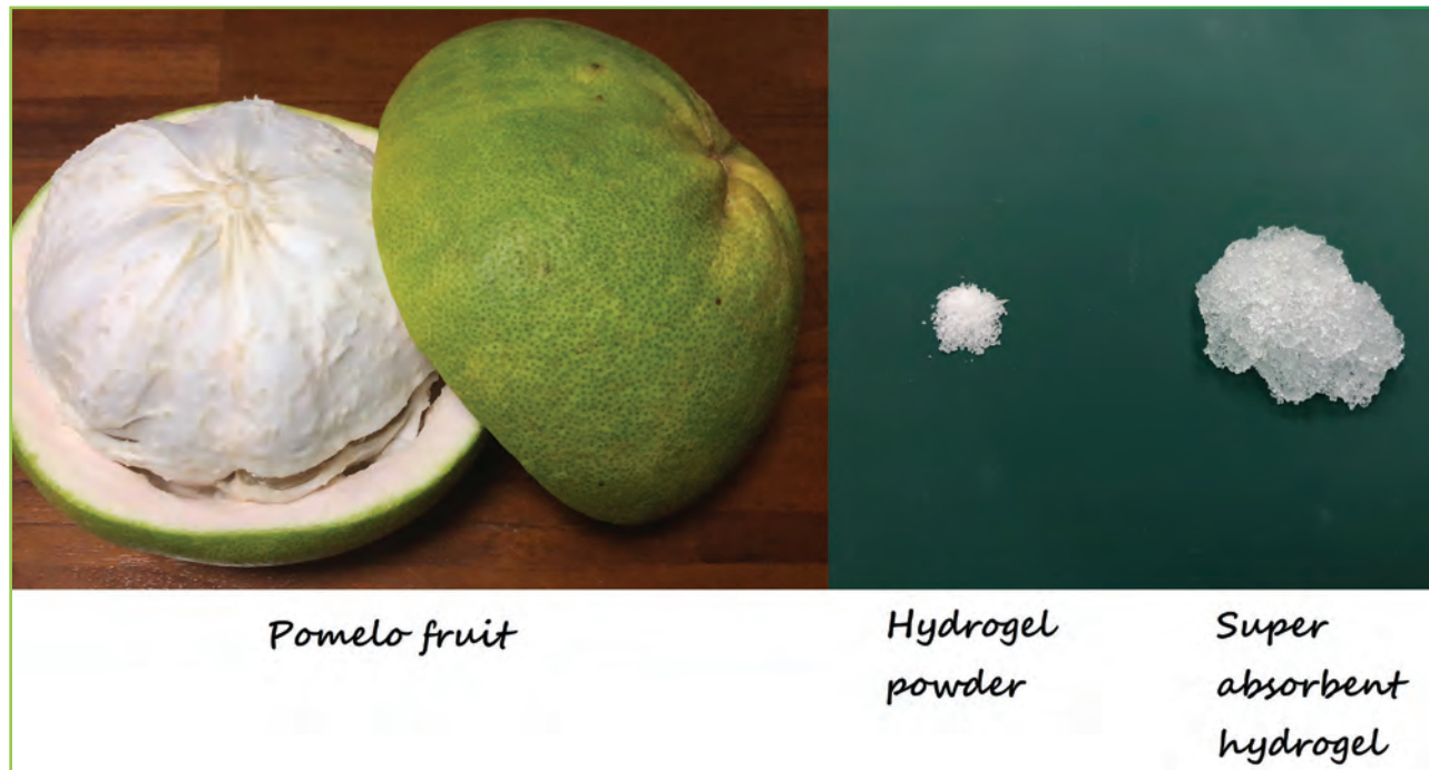
Pomelo peels converted into hydrogel powder with super absorbent property.
