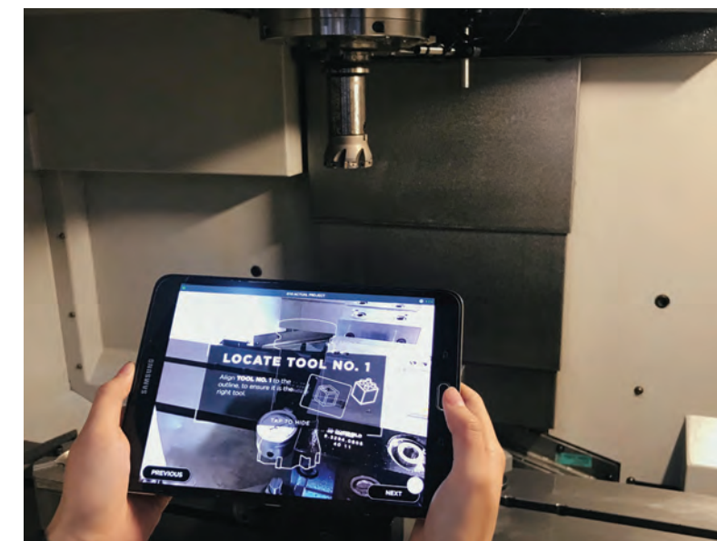
Digital Visualization (AR) for CNC machining operations: Guided instruction to locate the required tool.
