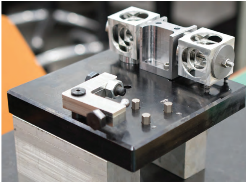
The actual fixture showing how the workpiece is loaded on the fixture for machining.
