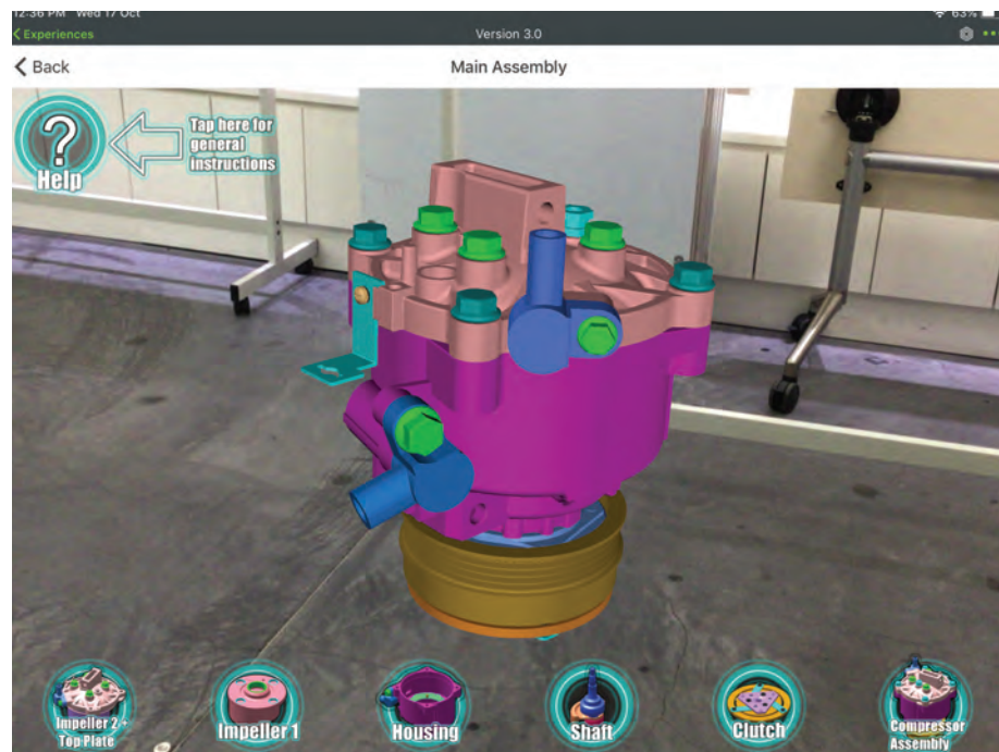
Main page of the instructional augmented reality app showing the overall compressor assembly.
